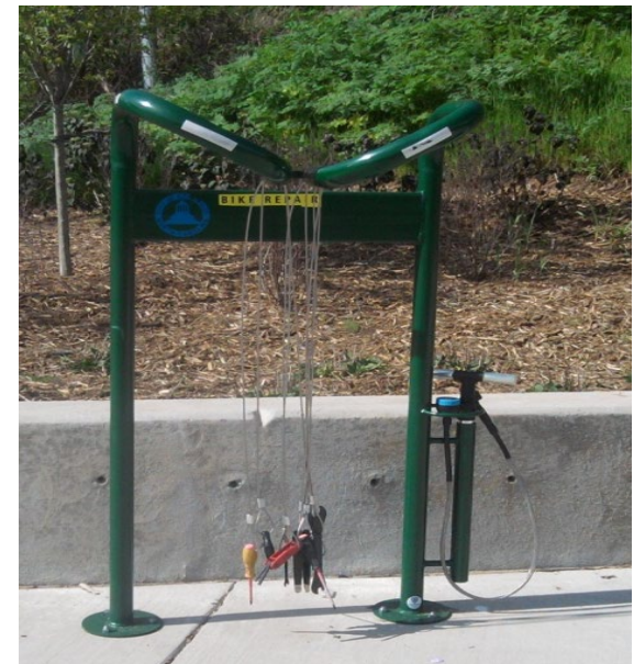
Example of Bicycle Fix-It (Public Repair) Station with Attached Pump and Tools.
