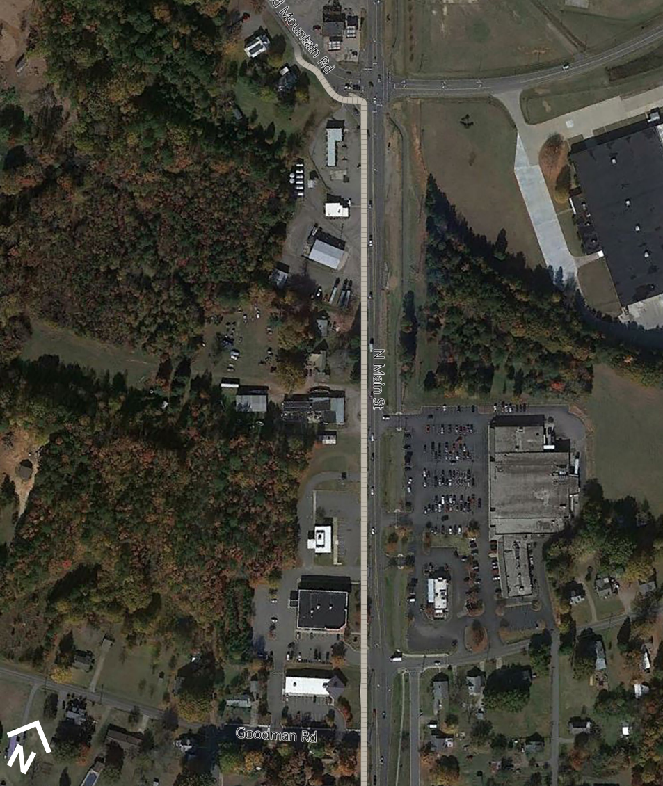
Aerial conceptual rendering of Project Ped-15, showing the proposed addition of the sidewalk along the west side of roadway.
