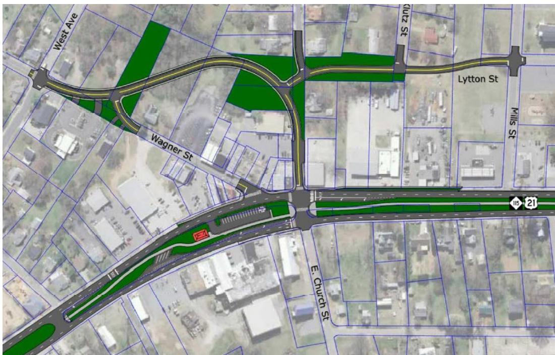
Figure 19 - Wagner Street and Main Street Intersection Recommended Realignment, US 21/NC 115 Corridor Mobility Strategy
