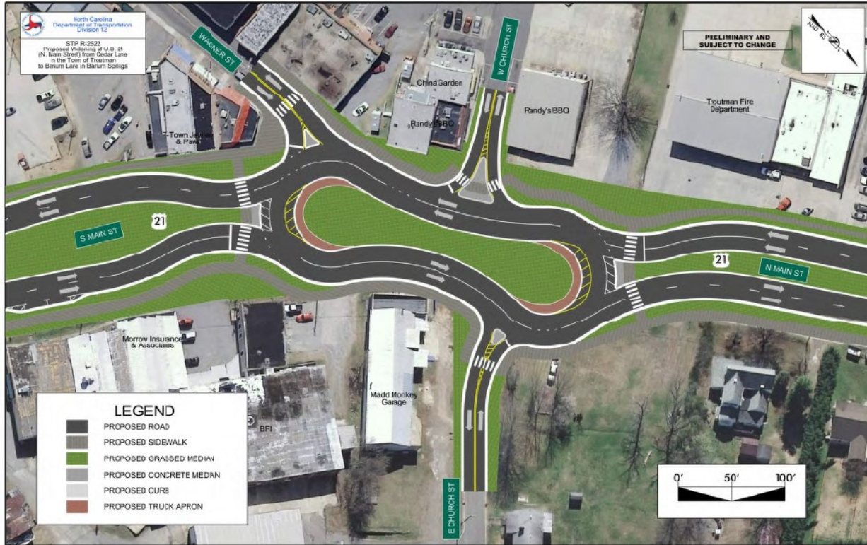
Figure 22 - Future R-2522 Peanut Shape Roundabout at Main Street/Wagner Street/Church Street, Source: NCDOT R-2522 Public Meeting Map 1 (Meeting Held May 2, 2019), https://www.ncdot.gov/news/public-meetings/Pages/R-2522-2019-05-02.aspx
